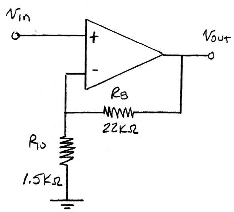
$$\frac{V_{OUT}}{V_{IN}} = \left(1 + \frac{R_8}{R_{10}}\right) \frac{1}{1 + \frac{1}{A} \left(1 + \frac{R_8}{R_{10}}\right)}$$
