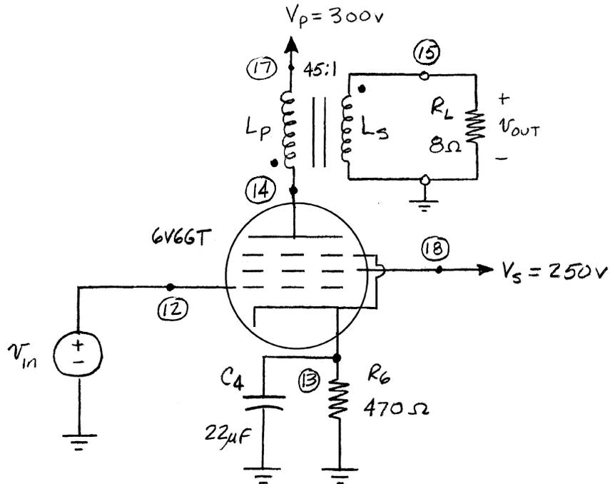
Pentode Power Output Stage (with by-pass)
